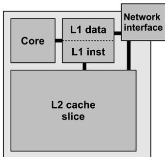
Fig. 3. Diagram of an individual tile.
