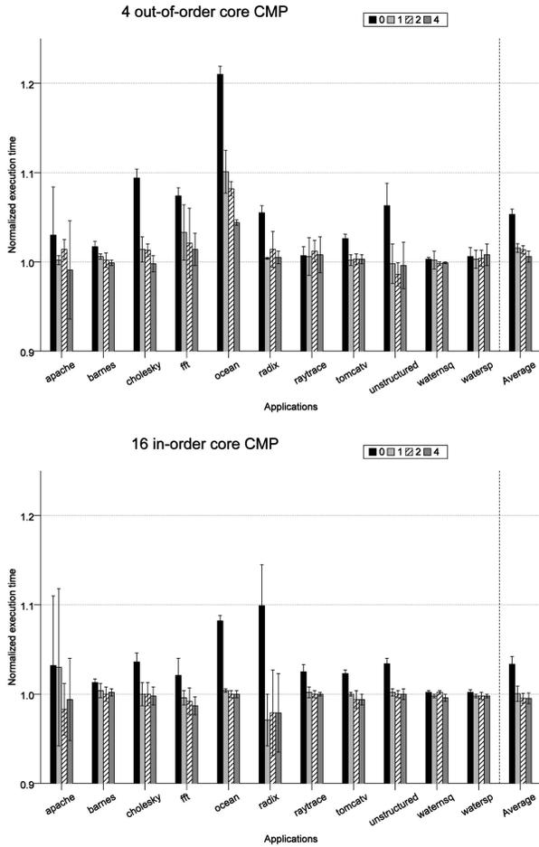
Fig. 4. Execution time overhead of our proposal compared to TOKENCMP for several backup buffer sizes.
